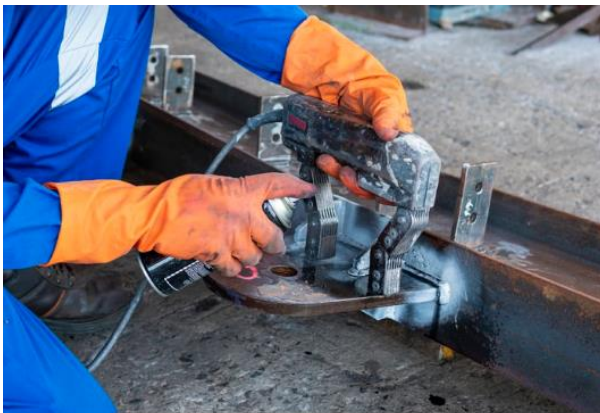
Figure 21: Magnetic particle inspection (NDE).
