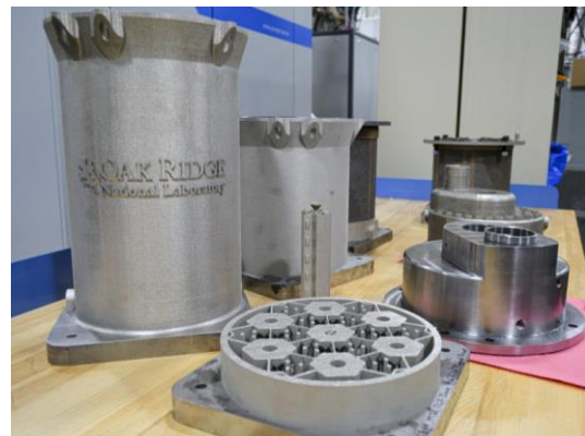
Figure 15: 3D-printed prototype nuclear reactor core. Credit: Brittany Cramer, ORNL, US Dept. of Energy [40].
