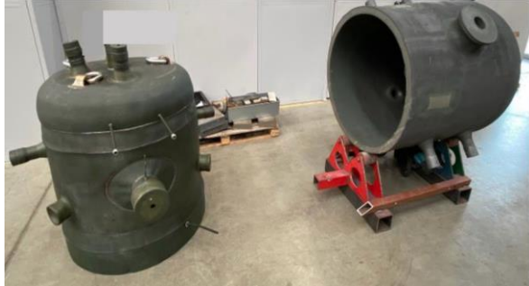
Figure 13: Small Vessel Demonstrator (SVD) – Upper and lower sections after HIPing. Image provided courtesy of Rolls-Royce © 2020 [35].
