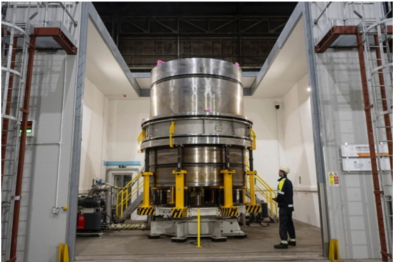
The reactor vessel welded by the new method
