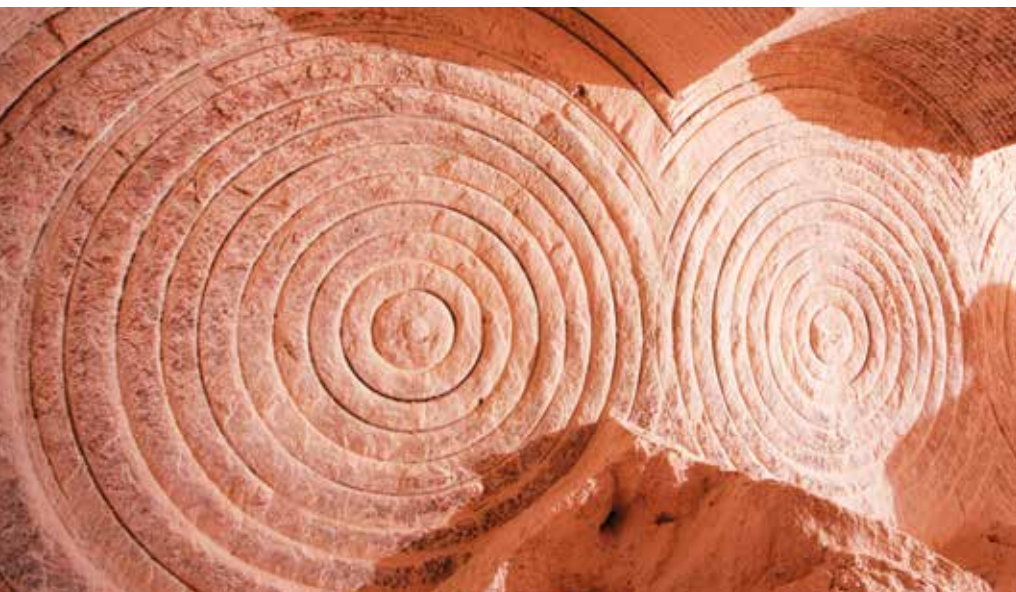
The signature marking created in a potash ore bed by a four-rotor underground mining machine. PHOTO COURTESY OF THE MOSAIC COMPANY.
